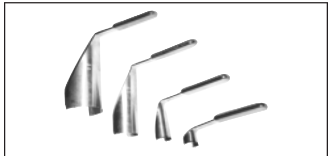
Figure 5.1B "C"-saw packing removal tool
